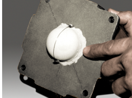
Cerabond™ 571 coats oxygen sensor.
