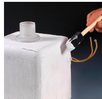
Ceramabond™ 569 bonds flex heater to quartz vessel.
