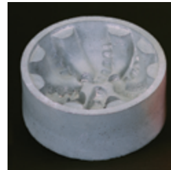
Ceramacast™ 673 mold for down-hole drill bit.
