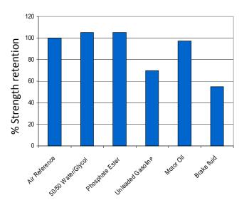
Specimens were immersed for 30 days at 85°C and tested at room temperature.
