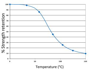
ET538 can withstand higher temperatures for brief periods (such as for paint baking and wave soldering processes) providing the joint is not unduly stressed. The minimum temperature the cured adhesive can be exposed to is -40°C (-40°F) depending on the materials being bonded.
